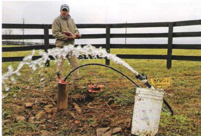
The flow of a well is measured by how many gallons per minute it produces
